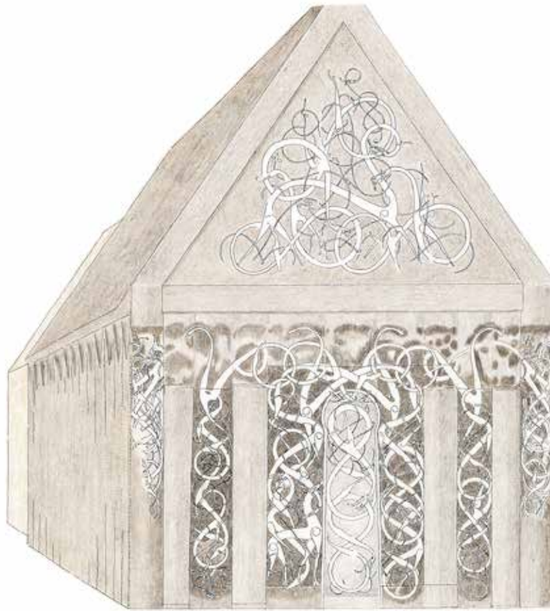
Krogh's reconstruction of the preceding church at Urnes based on the preserved reused materials and traces in these. Non-documented parts are shown without an outline.
