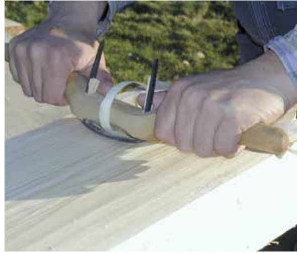
By trying out different tools and creating tool marks it becomes easier to understand the old traces. We find that the edge, and the humidity and characteristics of the materials affect the result. The picture shows a spoke shave that goes together with the hewing process. The more recent planes with a flat sole belong to sawing technology and modern carpentry. Photo: Kristen Åmodt 2002.
