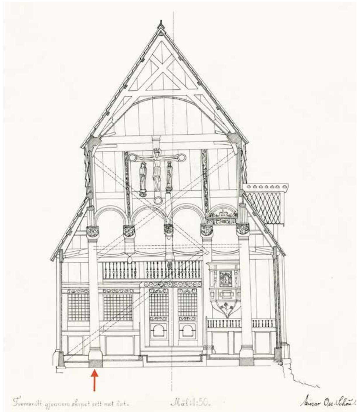
Elevation showing cross-section of the nave at Urnes stave church from the east. Subsidence on the church's north side is indicated by a red arrow. Drawing by Einar Oscar Schou. Undated.
